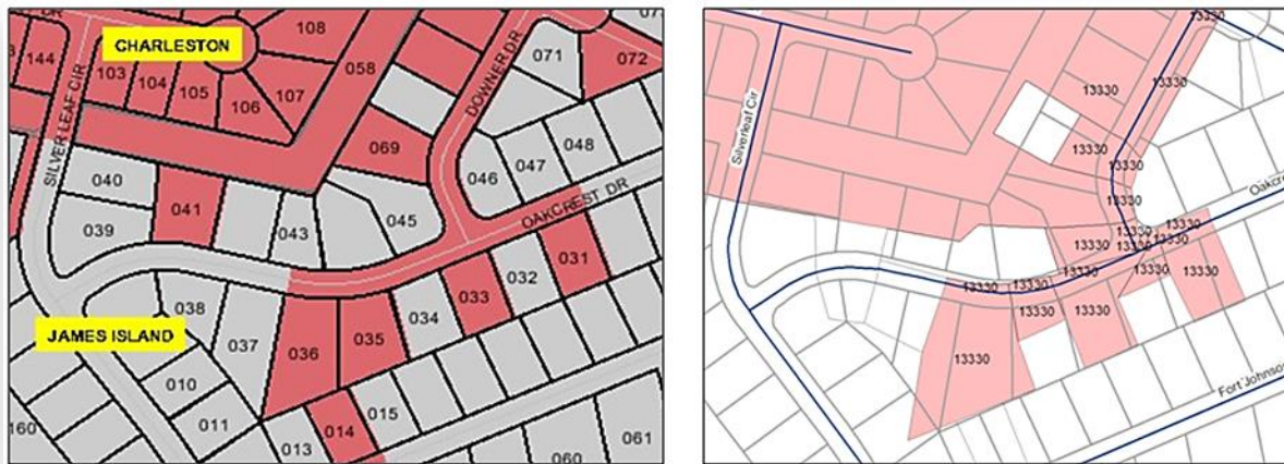
Figure 5 - Comparison of Charleston, SC, parcel-based boundaries (left) and the TIGER representation (right) showing the misalignment of these two data sources in the right side image. (Source: Cowen, 2011)
