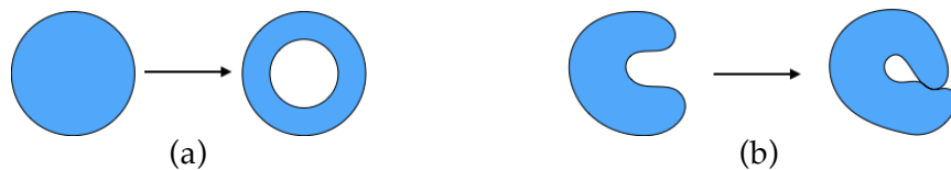
Figure 3: (a) Cutting a hole from an object, and (b) self-intersection of an object, both resulting in the same output: a ring.
